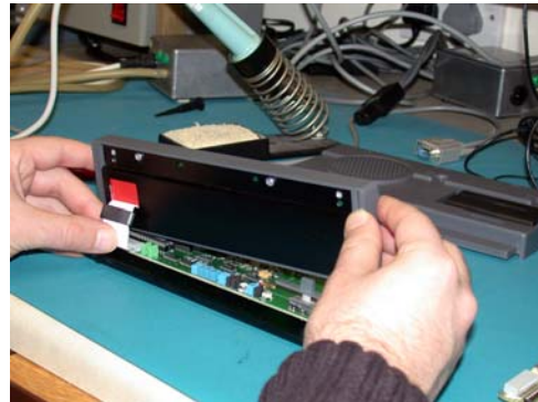
Fig. 1 – Fitting the MS20 Panel
