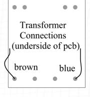
• Solder the IEC mains inlet onto the PCB with the brown and blue wires arranged as they were at the start.
