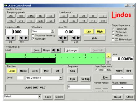
This panel shows the oscillator settings in the top half of the window and the measurement options and measured values in the bottom half. Many of the buttons and icons provide help if you move the mouse pointer over them and the help often gives details of keyboard shortcuts as well as explaining what they are for.
