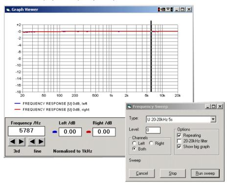
Frequency sweeps can be run as part of an automatic test sequence and most of the supplied test sequences include a frequency sweep test, but it is often more convenient to use the **Frequency sweep** menu, especially as it allows repeating sweeps.
