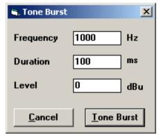
range 0.1 to 6553.5ms when controlling an LA100 or to a resolution of 1ms in the range 1-255ms on a MiniSonic.
